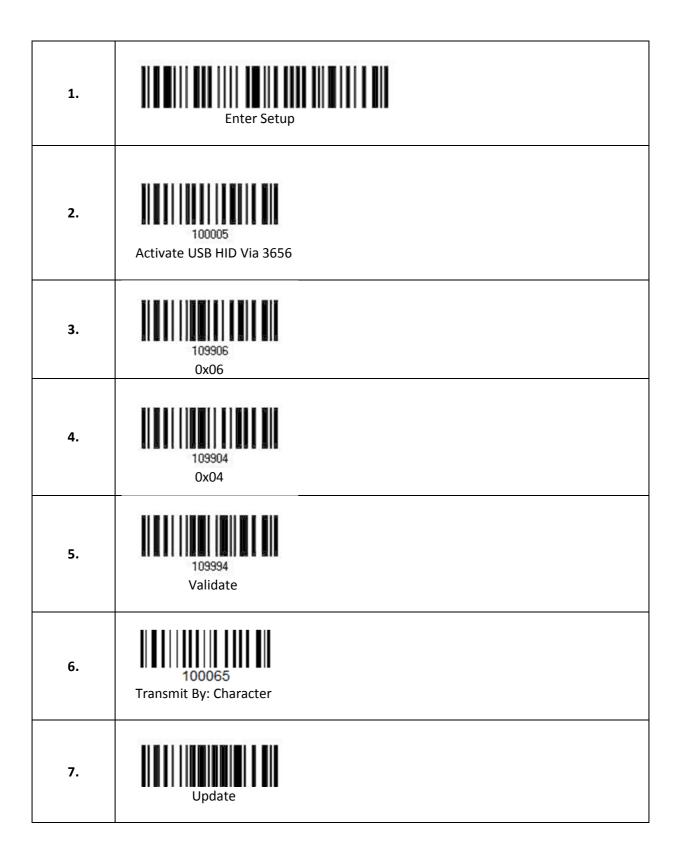
**Step 8:** After scanning the barcodes, you will notice a 3 beep sound indicating a successful link, also notice the Blue light on the cradle is still flashing approximately 5 times in 1 second, if not, please follow Step 3 to Step 8 again.
