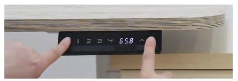
The screen will now display an 'S', Press the down button, the new minimum height will then display on the controller.
