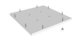
Step 4: On opposite side of Spinner Base panel (A) line up spinner plate with holes and push through bolts. Lock bolts in with 4 nuts (F).
