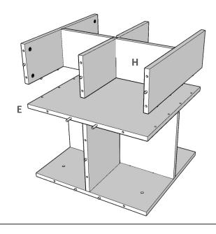
Step 7: Insert 12 cam pins (K) into both Side Panels (F). Push into sides of unit. Lock cam locks by turning until tight.
