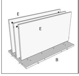
Step 4: Push side panels (D) into base panel (B). Lock cam locks by turning until tight.
