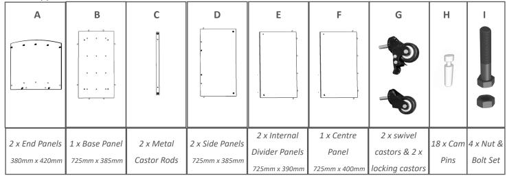
Step 1: screw all cam pins (H) into metal screw holes in (A) & (D)
