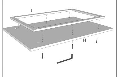
Step 8: Screw in 4 cam pins into other side of Base Panel (H) and then push onto frame. Lock cam locks by turning until tight.
