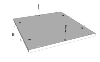
Step 2: Push Base Side Panels - Long (B) into Base Side Panels - Short (A) to make a box. Lock cam locks by turning until tight.
