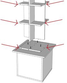
Step 18: Screw in acrylics onto outside of spinners using 40 x 9mm bolt (S). Don't overtighten as you will crack the acrylic.
