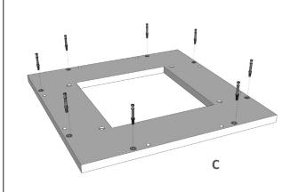
Step 4: Push Unit Base Panel (C) into Side Panels. Base Panel can go on either end. Lock cam locks by turning until tight.
