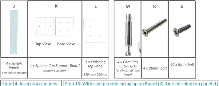
Step 14: Insert 4 x cam pins (M) into Spinner Top Support Board (K).
