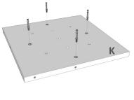
Step 16: Push top of spinner onto Dividers Boards. Make sure holes on side of all panels line up and are on the left side. Lock cam locks by turning until tight.
