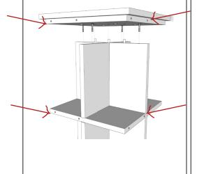
Step 17: With 2 people. Lift top of spinner onto assembled base. Make sure holes on outside line up. Lock cam locks by turning until tight.
