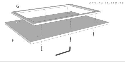
Step 6: Screw in 8 x cam pins (I) into Base Panel (F). Connect base panel (F) to bottom of unit. Lock cam locks by turning until tight.
