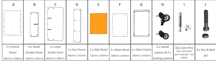
Step 1: Make 2 internal shelves. For each shelf, screw 8 x cam pins (I) into 2 x Face Panels (D). Push into 2 small divider panels (B). Lock cam-locks by turning until tight.
