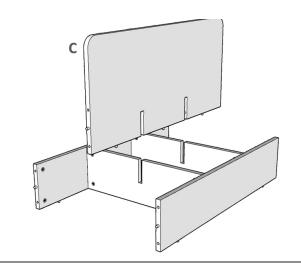
Step 3: Add 4 x cam pins (I) onto centre panel (A). Push panel A onto base of 1 x internal shelf (previous step). Lock cam locks by turniing until tight.
